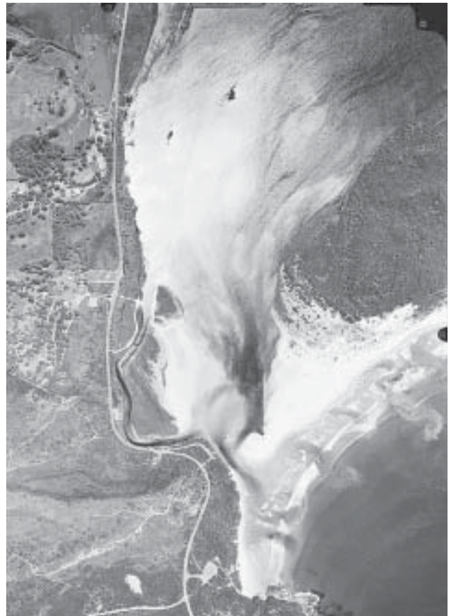
Figure 10: Bar in November 1996 showing multiple rip cells, narrow beach in front of SLSC and migration of the bar channel from opening position of 100 m.
